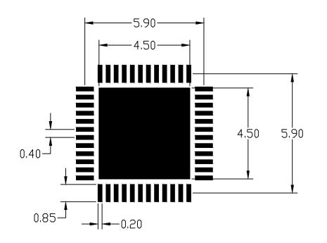
PKG, CDDES [T4866-1 / T4866+1] [T4866-1C / T4866+1C] [T4866N-1 / T4866N+1] [T4866-2 / T4866+2] [T4866-2C / T4866+2C] [T4866-3 / T4866+3] [T4866-3C / T4866+3C] [T4866MK+2] [T4866+4]
